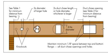
Knockouts are prescored holes provided for the contractor's convenience to install electrical or small plumbing lines. They are 1-1/2 inches in diameter, and are spaced 15 inches on centre along the length of the I-joist. Where possible, it is preferable to use knockouts instead of field-cut holes.
